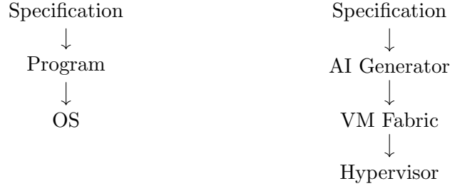
Figure 1: Comparison between conventional systems and VM Fabric. The proposed architecture replaces static programs with dynamically generated execution structures.
